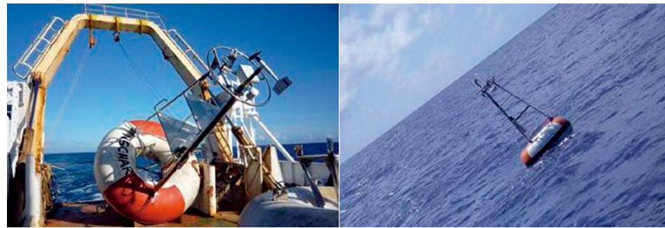
Fig. 1. The deployment and recovery of the ATLAS moorings.
