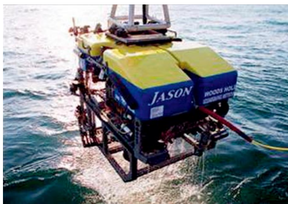
Fig. 4. The design prototype for TORI self-developed ROV: JASON II by WHOI.
