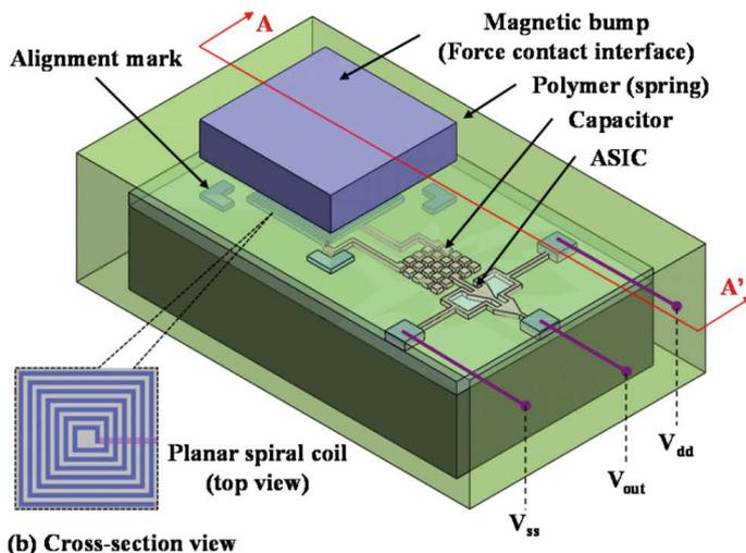
▲ The first non-suspended CMOS tactile force and ASIC sensor SoC
