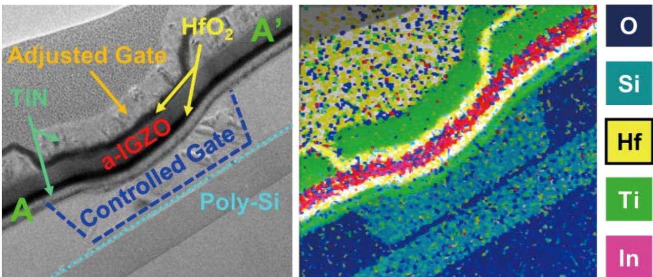
▲ Heterogeneous IGZO/poly-Si stacked complementary field-effect transistor structure
