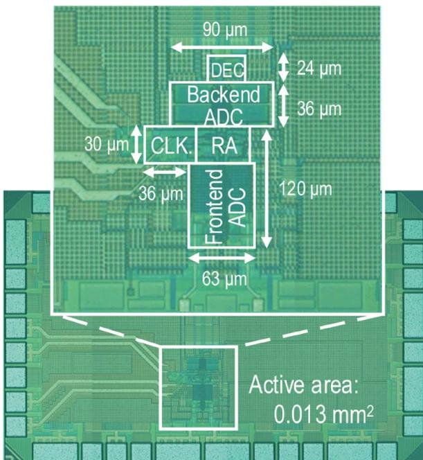
▲ High-resolution 130MSPS pipelined SAR ADC
