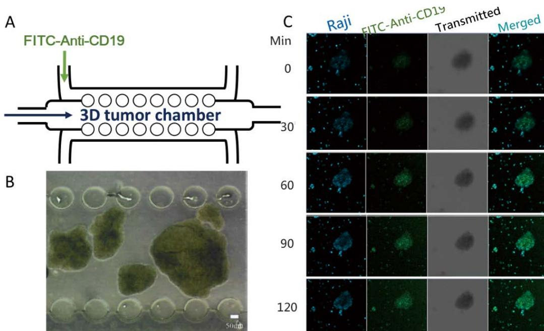
▲ Tumor-on-chip for testing antibody infiltration
