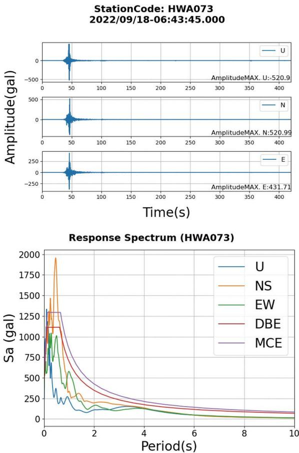
▲ An example of acceleration waveforms and response spectra observed by a strong motion station
