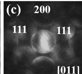
▲ The selected area diffraction pattern of Ge (100)/Si (100) and the converged beam electron diffraction patterns of (b) Ge (111) and (c) Ge (100)
