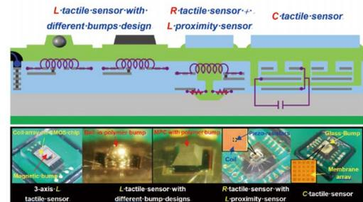
▲ CMOS-MEMS tactile sensors
