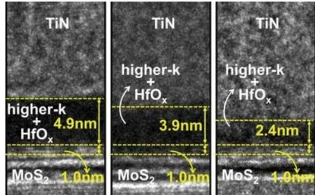
▲ Record for thinnest effective oxide layer in ultrathin dielectric film produced on a 2D material
