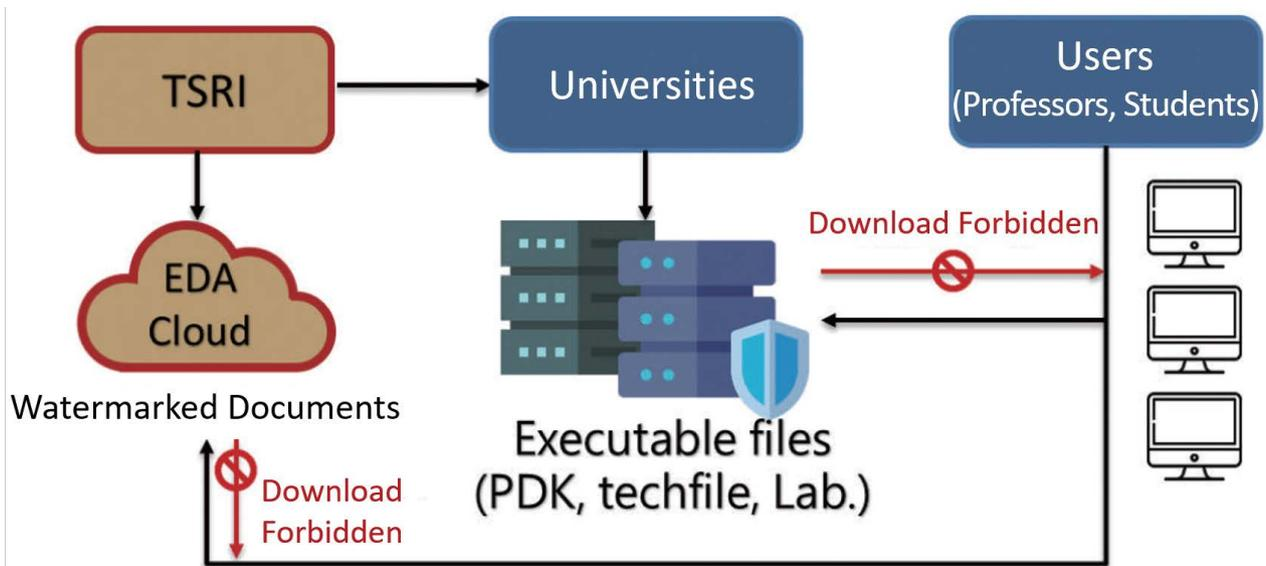
▲ N16 ADFP information security structure with unidirectionality to ensure security of sensitive process data
