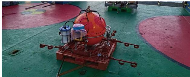
▲ Deployment of ocean bottom seismometer (OBS) and ocean bottom electro-magnetometer (OBEM) from the University of Tokyo results in new milestone for seafloor observation instruments
