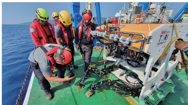
◀ 海洋中心與中山大學合作研發之輕型工作級 ROV Light Work-Class ROV developed by TORI and National Sun Yat-sen University
