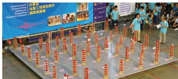
▼ Models were tested on a shaking table
