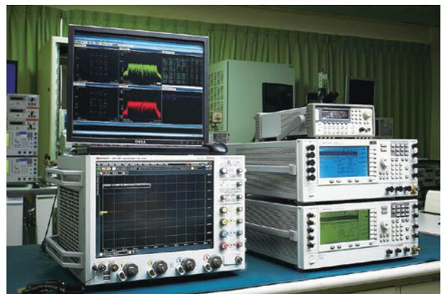
▼ Millimeter wave multichannel transceiver measurement system
