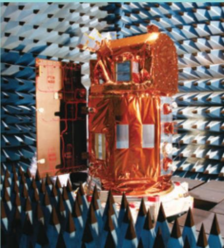
FORMOSAT-5 is the first optical remote sensing satellite made in Taiwan. The satellite system was fully assembled in 2015 and underwent a series of stringent tests such as the comprehensive performance test, satellite end-to-end tests, space and launch vehicle environments tests. The satellite system is now fully prepared for launch, which is scheduled to take place in the third quarter of 2016.
