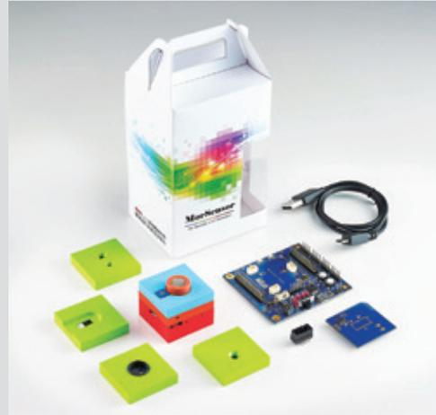
▼ MorSensor wireless sensor bricks
