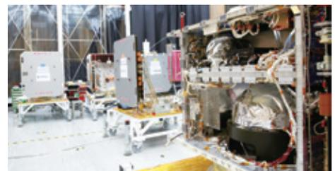
▼ Assembly and testing for FORMOSAT-7 mission satellites
