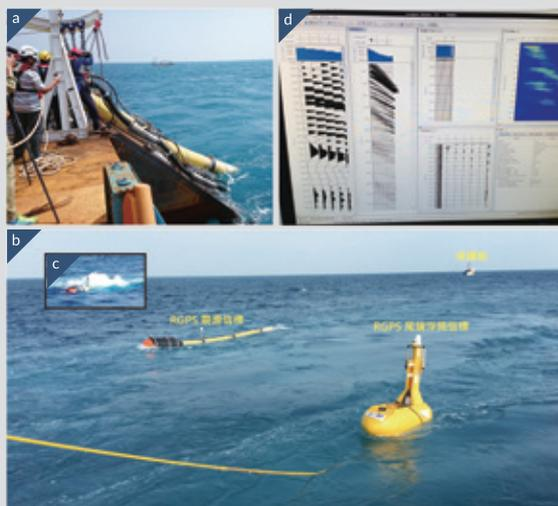
▼ Sea trial of Large-offset Multi-channel Seismic System; (a) Deployment of the seismic source array; (b) Seismic source with precise GPS (RGPS) (left) and tail buoy (right) in operation; (c) Onsite shooting by the seismic source array; (d) Seismic data acquisition
