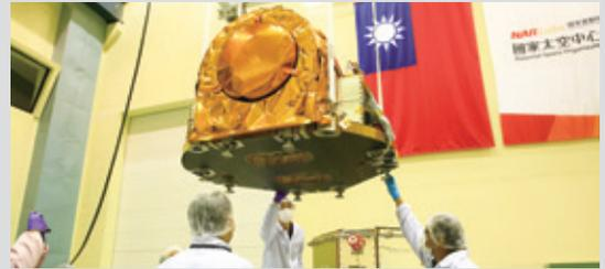
▼ Assembling the FORMOSAT-5 satellite optical remote sensing instrument and spacecraft
