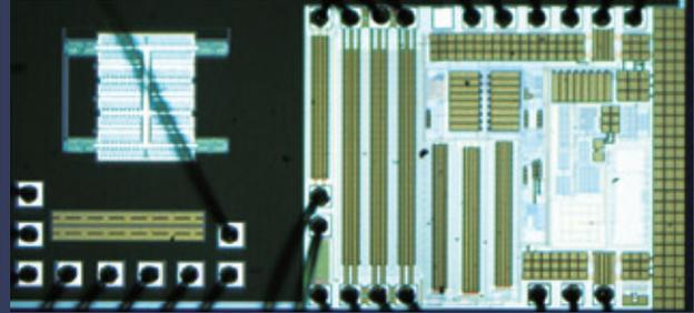
▼ Silicon MEMS oscillator and clock generator
