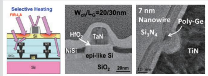
▼ The selective heating technology using far-infrared laser was adopted to realize a sub-10nm stackable transistor
