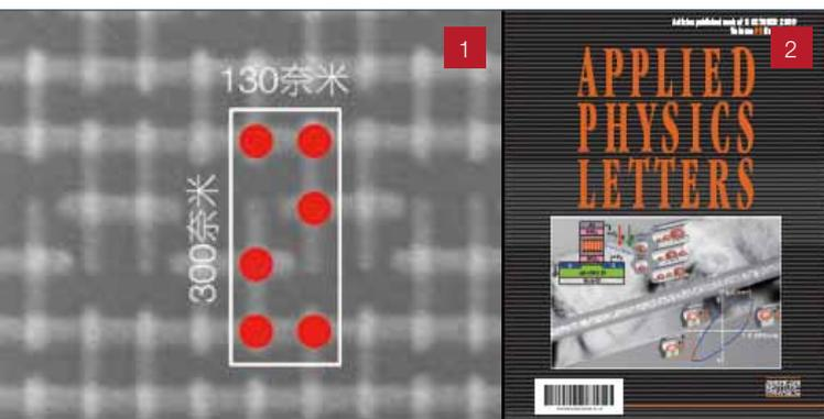
1 The 16nm node device (i.e. static random access memory or SRAM) developed by the NDL. As many as six transistors are located within the white box, which translates to a density of 15 billion transistors per  $\text{cm}^2$ . The capacity of such a device is approximately 10x that of the existing 45nm device and the power consumption is expected to be reduced by half. 2 Selected as the cover story for the renowned physics journal, Applied Physics Letters.
