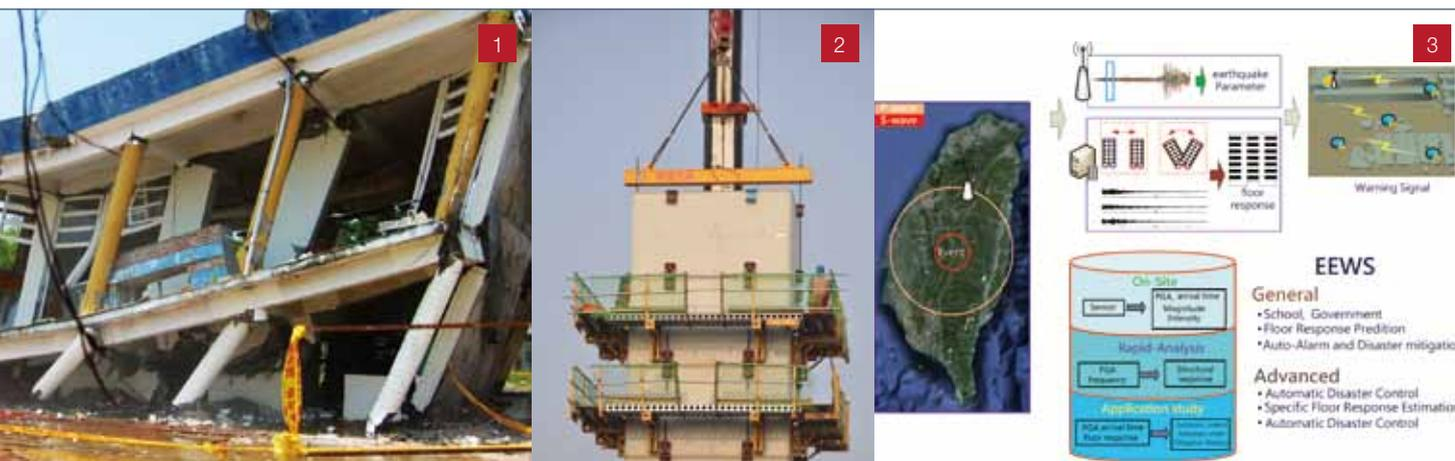
1 In-situ experiment of existing school building 2 The precast segmental post-tensioned concrete bridge column 3 Diagram of Earthquake Early Warning System (EEWS)
